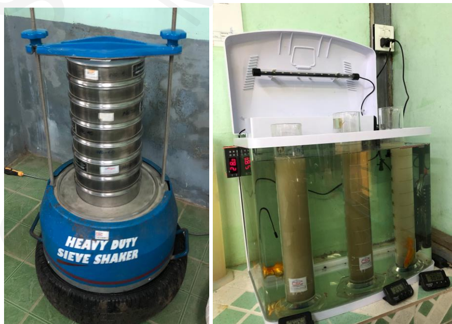
Figure 67: Sieve Analysis and Hydrometer Analysis
