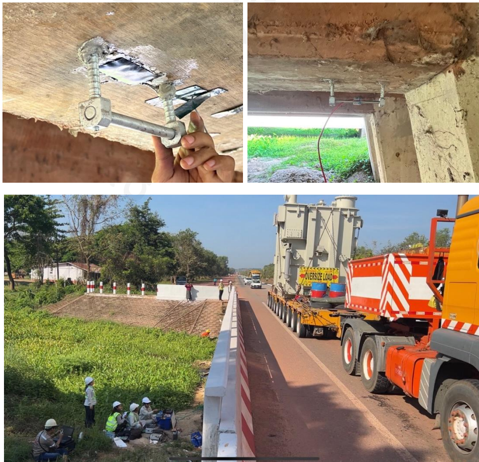
Figure 46: Stress Monitoring at Vehicle Bridge
