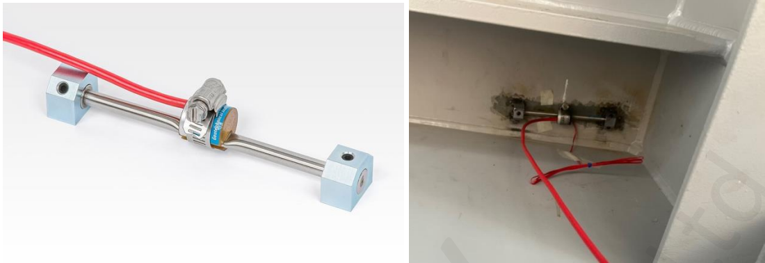
Figure 32: VW Arc Weldable Strain Gauge and Sample Welded to I-Beam
