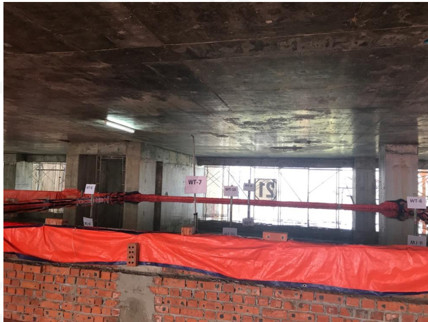
Figure 42: Floor/ Slab Load Test
