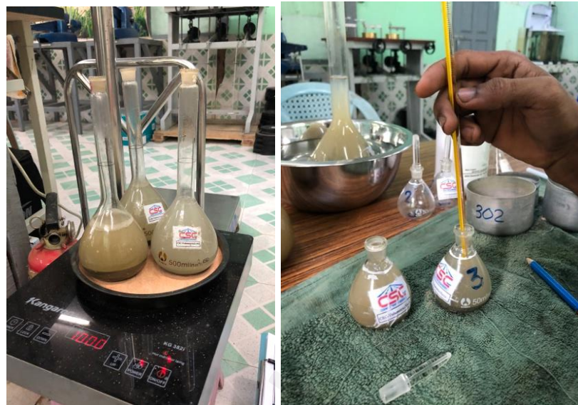
Figure 66: Specific Gravity Testing of Samples
