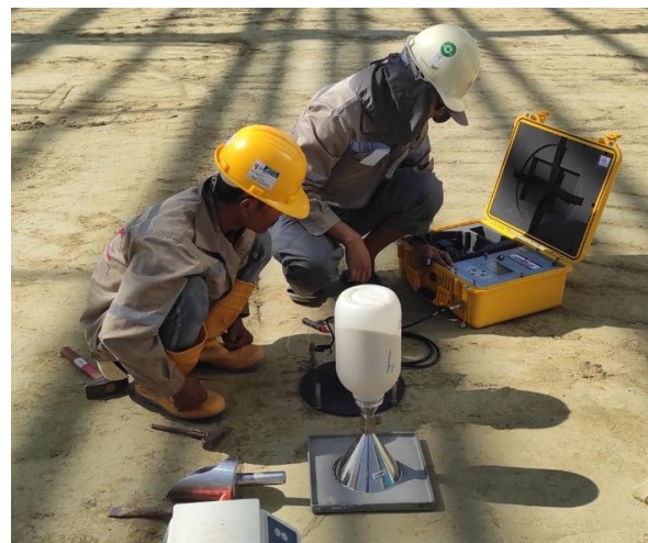
Figure 24: EDG Tests Soil Model Building with Sand Cone Test
