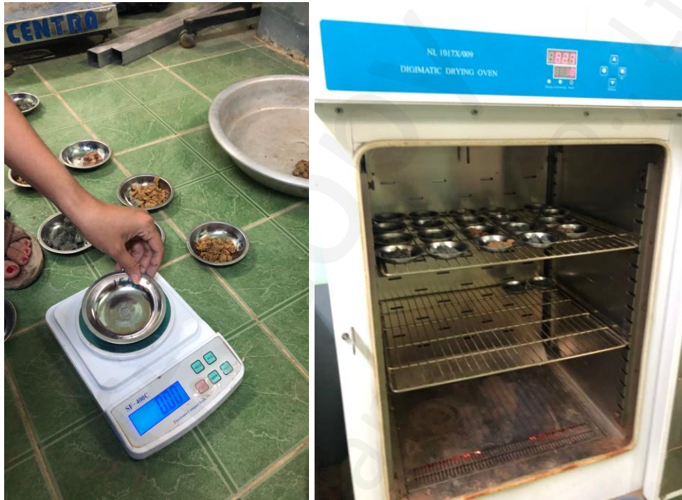
Figure 65: Moisture Testing of Samples
