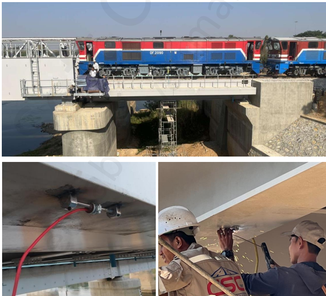
Figure 48: Load Test for Railway Bridge
