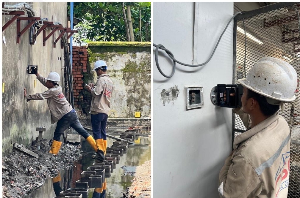
Figure 29: Adjacent Structures Tilt Monitoring
