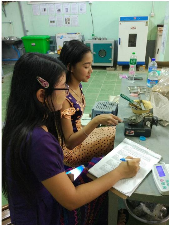
Liquid Limit Determination Test
