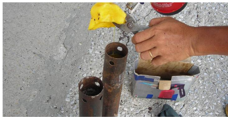
Undisturbed Samples taking process
