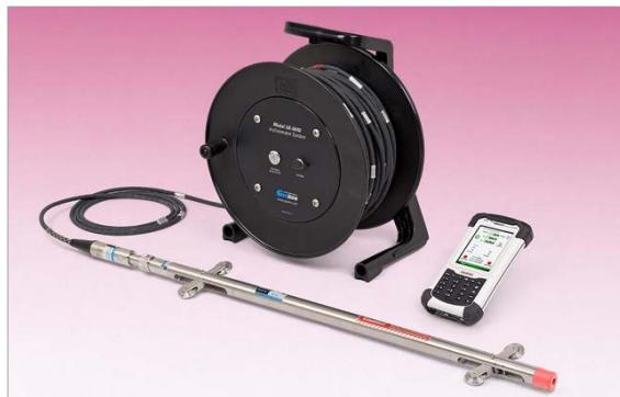
Inclinometer Reading Instruments
