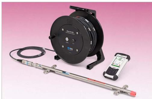
*Inclinometer Reading Instruments*
