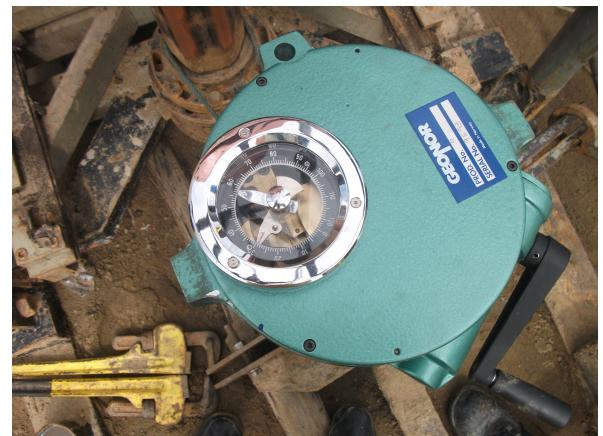
*Vane Shear Test*
