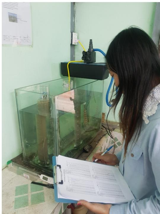
Hydrometer Analysis Test
